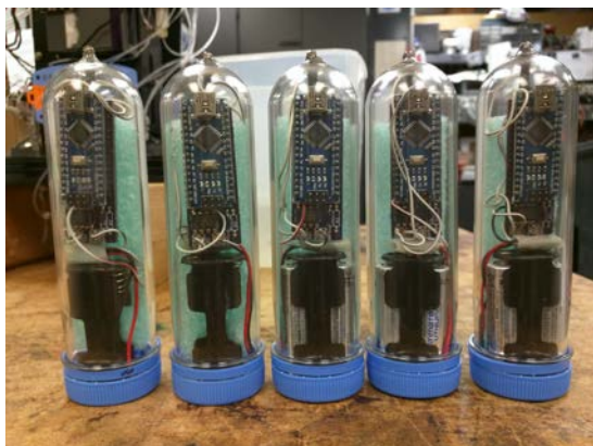
Figure 6: Picture of the low cost, long term, submersible temperature data loggers.
