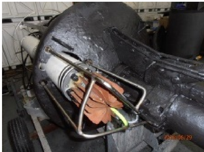
Figure 1: A picture of the new blue wavelength in-line spectrometer mounted on the MOBY buoy for the August 2016 deployment. The spectrometer is being used along with the heritage optical system for testing. In November 2017 we will be installing a full blue and red system to begin a one-year cross-over experiment with the heritage MOBY optical system.
