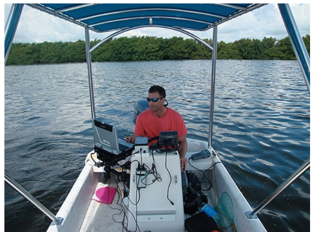
Figure 1: Image of the survey skiff used to collect geo-referenced images of the bottom at near-shore benthic habitats of Biscayne Bay
