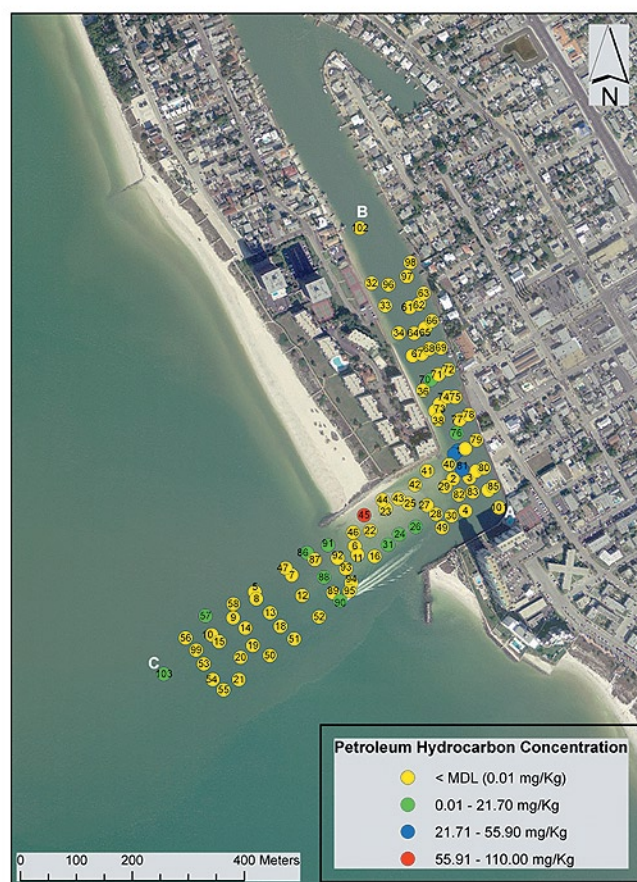
Figure 5: Blind Pass, Tampa Bay, Florida. Sediment cores petroleum hydrocarbon concentrations (C8-C40) at 200-299 cm core intervals. Note the number of samples below detection, with a few higher values resulting in a “patchy” petroleum hydrocarbon distribution. Over 100 cores were collected for characterization of petroleum hydrocarbons by Dr. Ping Wang and map created by Tanya Beck (USE, 2008).
